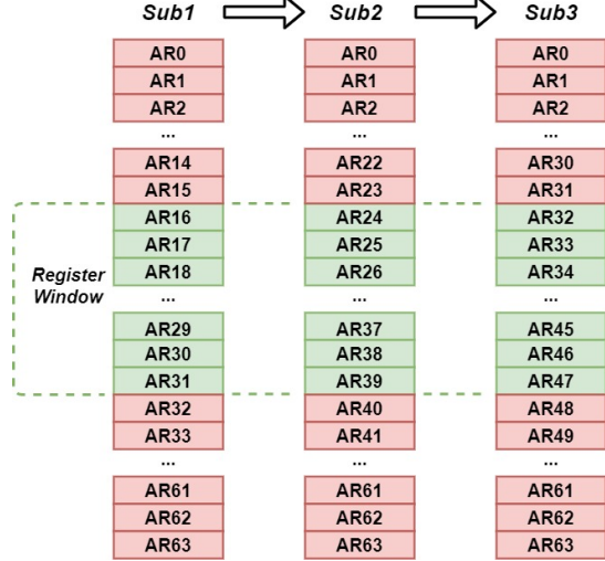
Fig. 1: Overview of the ESP32 register file. A subroutine only has access to the registers contained within the register window.
